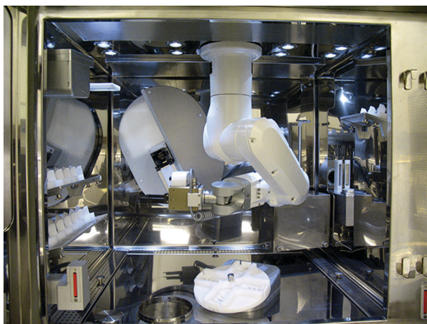
Figure A3.1 Robotics used for sterile compounding at Brigham and Women's Hospital.
